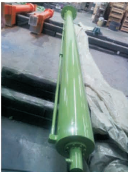
6550mm hydraulic cylinder uses 19 series
