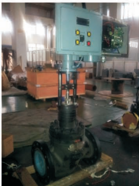
Automatic Control Valve use 17 series
