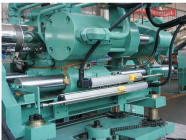
Multi-color plastic second injector
