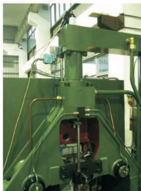
Hot chamber die-cast machine used Germanjet 17 series
